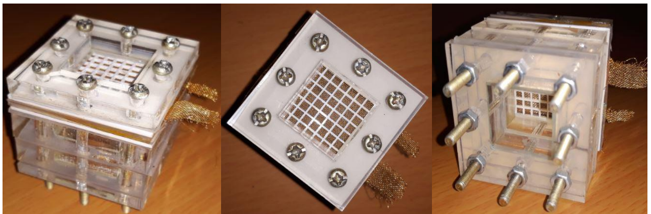
Fig. 4 Schematic view of the fabricated methanol micro-fuel cell
