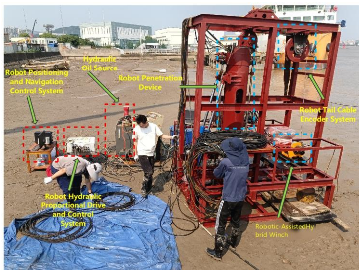
Figure 6. Robot and base station system test on the wharf tidal flat.
