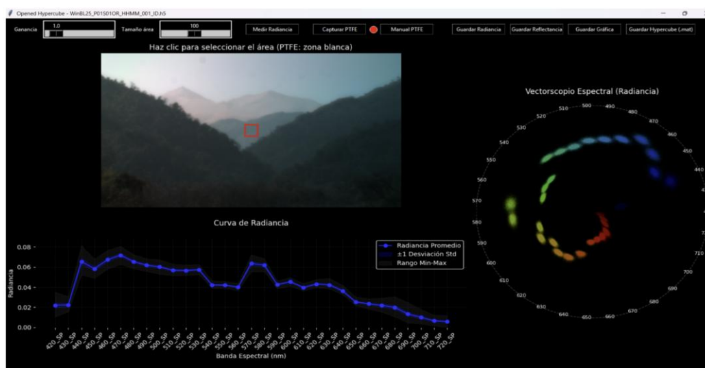
Figure 6. Interface of the hyperspectral analysis software used for data visualization and processing. In the upper left, the scene image is displayed with the selected area of interest (red rectangle), corresponding to the analyzed region. In the lower left, the average spectral radiance curve of the selected area is shown as a function of wavelength, together with the standard deviation and minimum–maximum range. On the right, the spectral vectorscope is displayed, representing the chromatic distribution of radiance in angular coordinates associated with wavelength.
