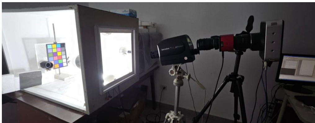
Figure 7. Experimental setup for spectral data acquisition, consisting of a controlled illumination booth containing a color chart and black and PTFE samples inside.
