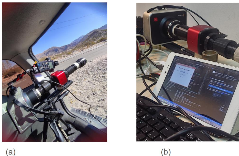
Figure 12. (a) Hyperspectral system mounted inside the trunk of a car for field measurements. (b) Image of the hyperspectral system being controlled via a computer tablet.
