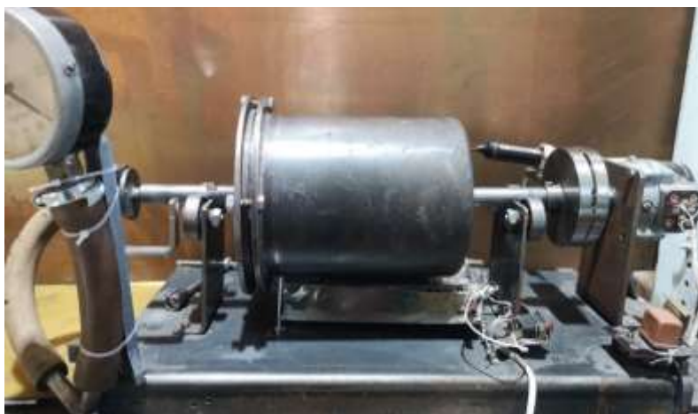
Figure 2. Reactor setup for gas-phase deposition of phosphate-based insulating coatings on iron powder particles under controlled temperature and reduced pressure conditions.
