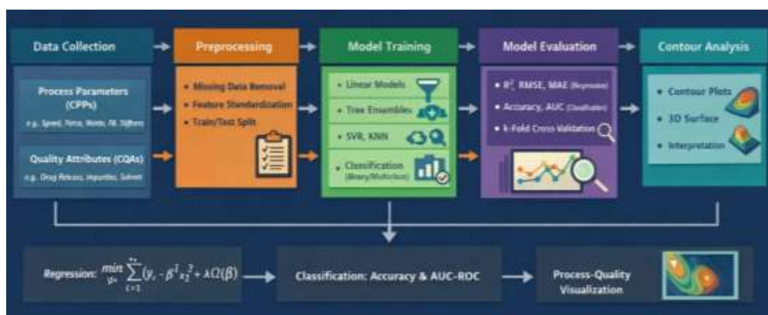
Figure 1. Methodological framework for machine learning–based prediction and process–quality exploration in pharmaceutical manufacturing. The workflow illustrates the sequential steps from batch-level data acquisition of critical process parameters (CPPs) and critical quality attributes (CQAs), through preprocessing (data cleaning, feature standardization, and train–test splitting), to supervised model development using regression and classification algorithms. Model performance is evaluated using cross-validation and hold-out metrics, including R^2 , RMSE, MAE, accuracy, and AUC. The trained models are subsequently used for feature importance
