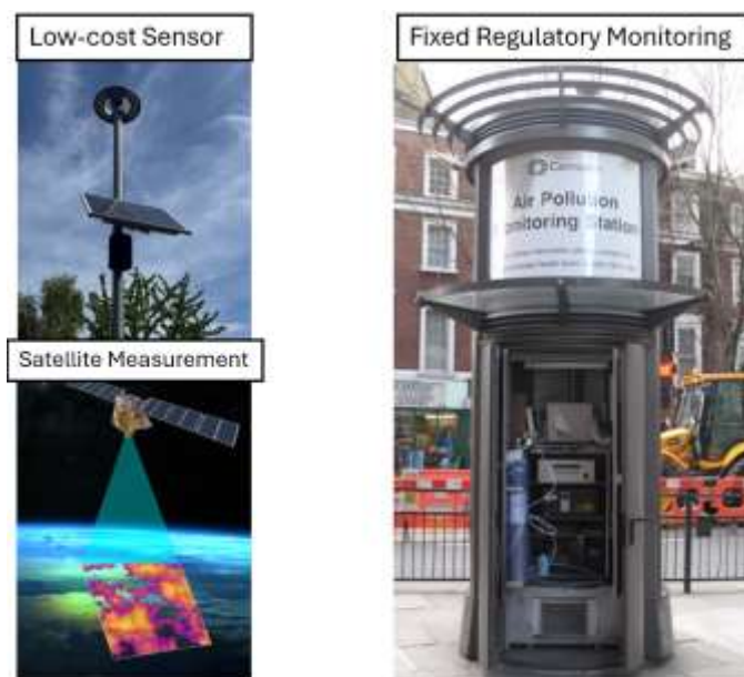
Figure 4. - Air Quality Measuring Systems.
