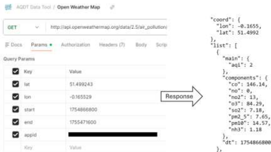
Figure 7. – Example of an API call and JSON response.
