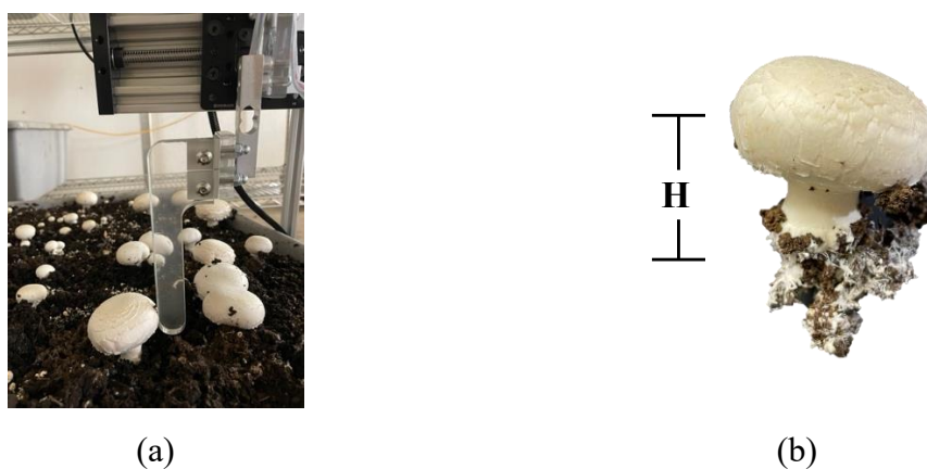
Figure 8. Experiment setup of the mushroom bending force measurement system: (a) Experimental setup in a real environment, showing the bending force applied to the mushroom until the cap touches the compost. (b) Height measurement between the point of contact with the bending finger and the mushroom base after the bending process.
