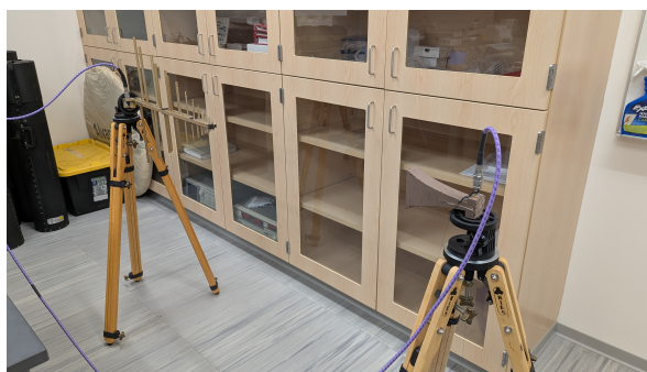
Figure 5. The co-polarized configuration to measure the radiation pattern of the printed RF horn.
