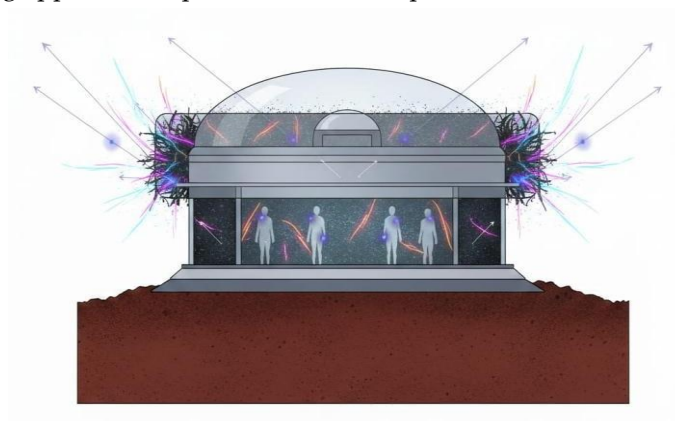
Figure 6. Melanin-based coating on habitat envelope: Space habitat section showing a melanin coating absorbing radiation.
