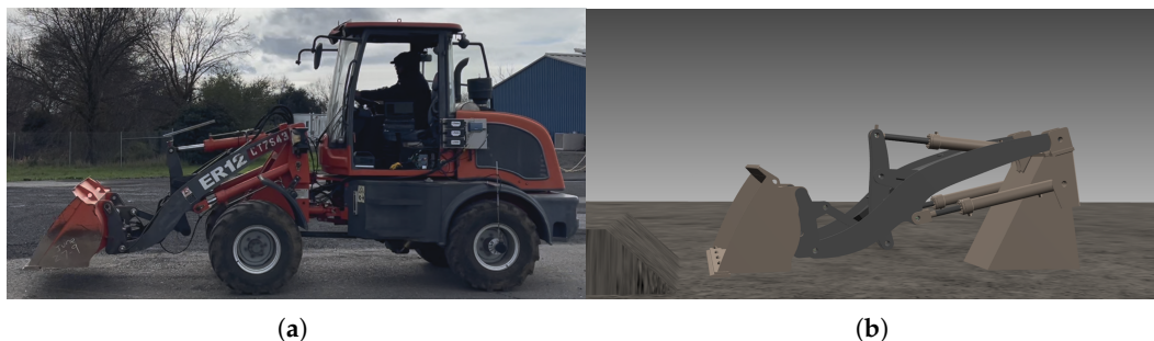
Figure 2. Wheel loaders available to develop the input duty cycle including: (a) AHMCT ER-12 wheel loader and (b) Algoryx digital-twin simulation.
