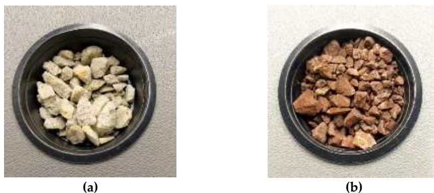
Figure 2. Types of substrates: (a) Artificial foamed-glass medium (GrowPlant); (b) Natural zeolite from the Shankhanai deposit.
