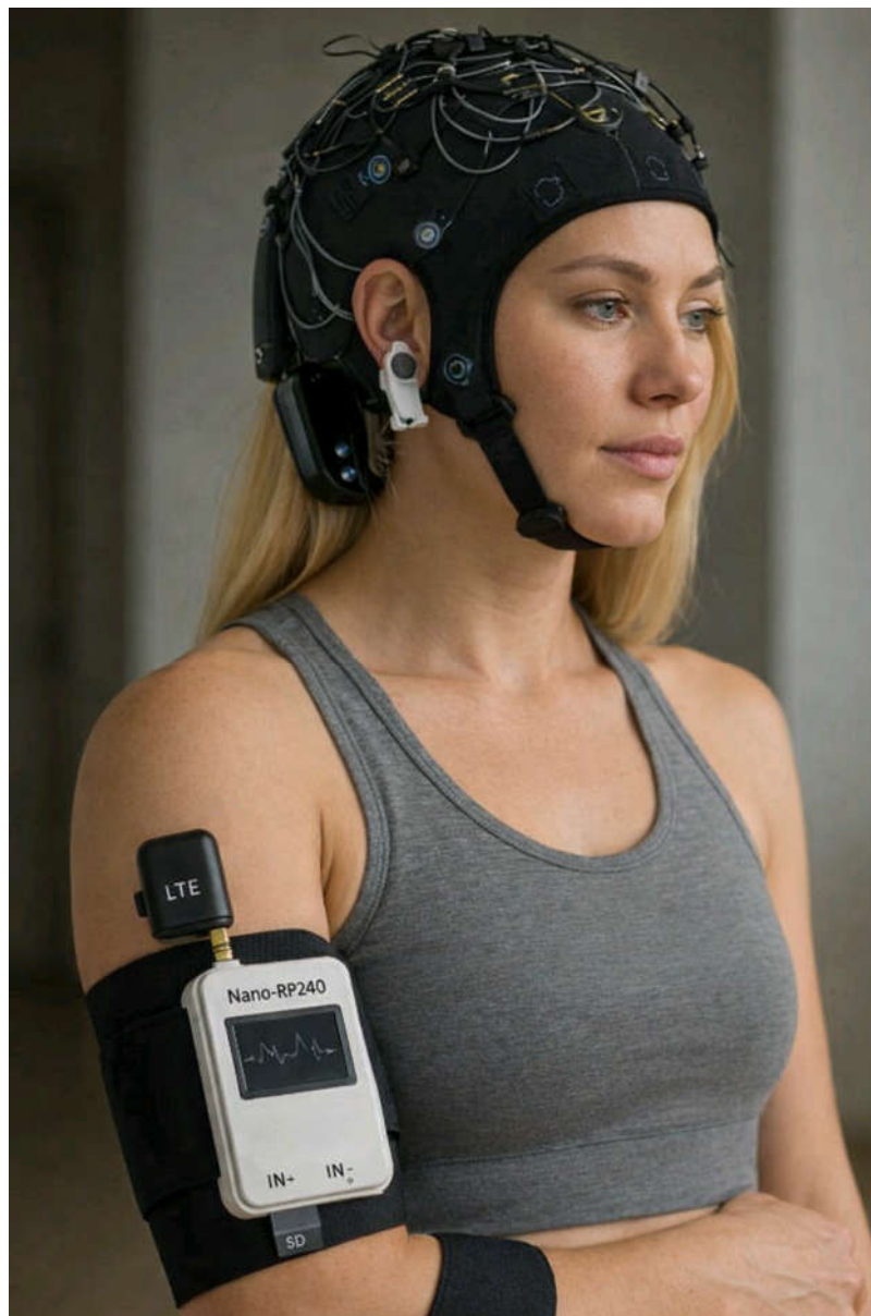
Figure 6. Mock-up illustration of the wearable composed of a headcap having BCI biosensors integrated into an arm-mounted form factor with LTE connectivity and hot-swappable external storage.
