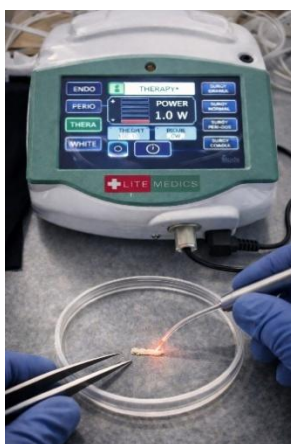
Figure 2. Experimental setup for dental laser application under controlled laboratory conditions. A Lite Medics laser unit was operated in therapy mode at an output power of 1.0 W, delivering focused laser energy to a tissue-like sample positioned in a sterile Petri dish and stabilized with precision forceps, illustrating laser–tissue interaction in a simulated clinical environment.
