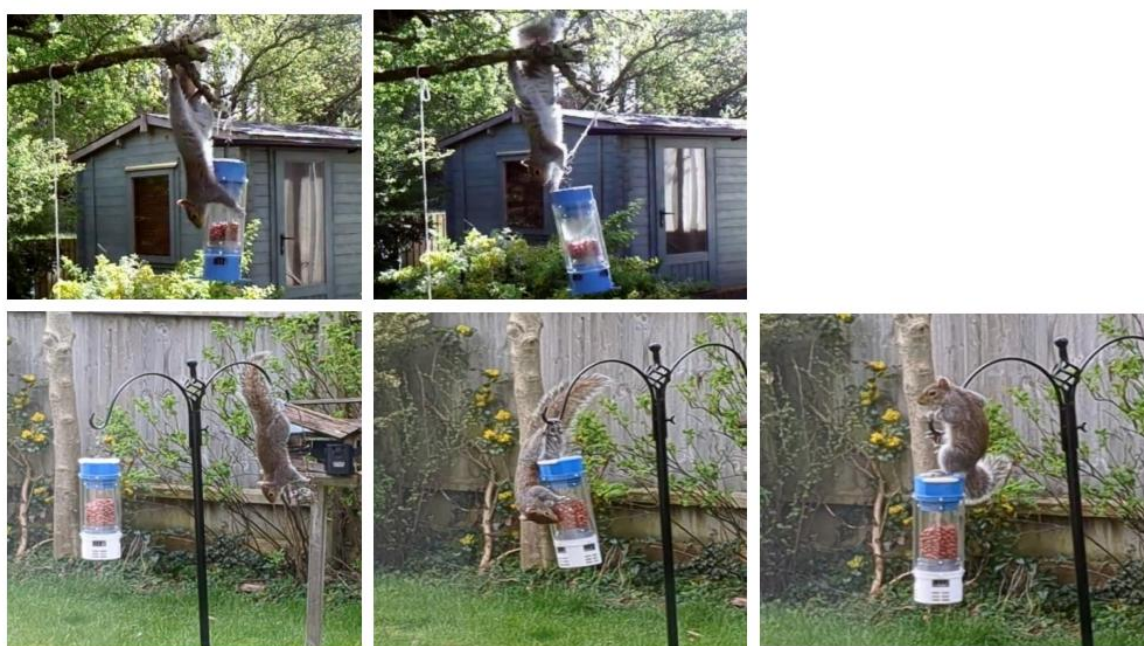
Figure 5. Maneuvering positions of squirrel on the protruding cantilever design and ladder-like design.
