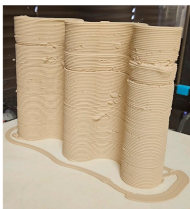
Figure 2. Printed clay wall specimen showing intentionally introduced defects including voids, bulges, and irregular layer heights.
