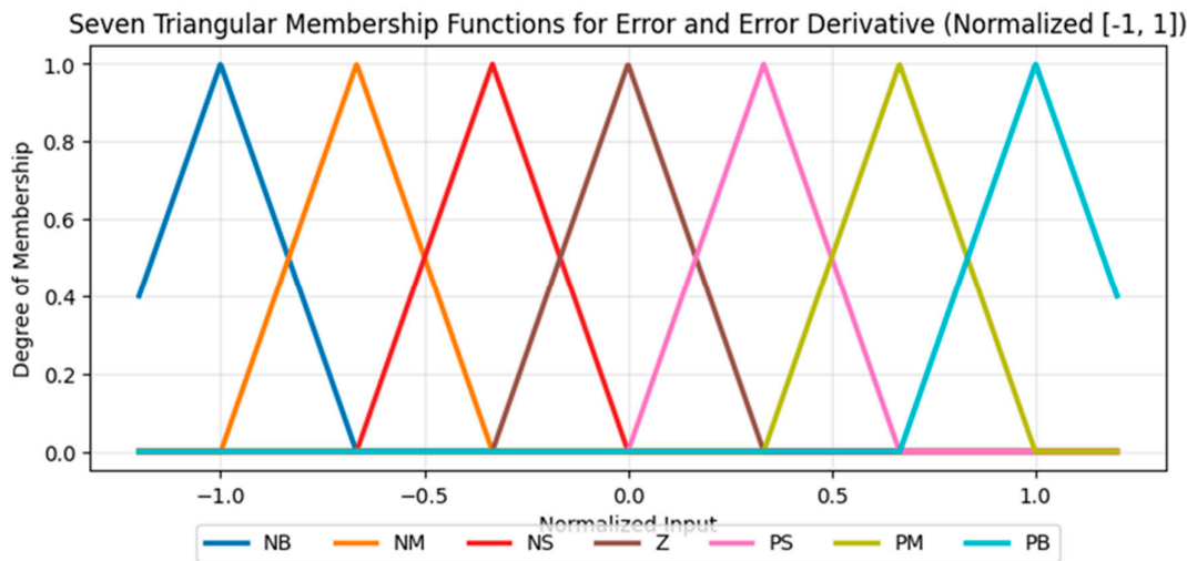
Figure A1. Seven symmetric triangular membership functions with 50% overlap (NB, NM, NS, ZE, PS, PM, PB) are uniformly distributed over the normalized universe of discourse [-1, 1] for both e_n and \dot{e}_n , following the standard industrial practice [8,22].
