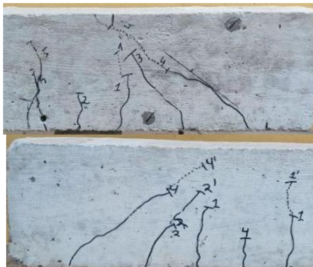
Figure 4. Formation of shear cracks in samples from the S2 series.
