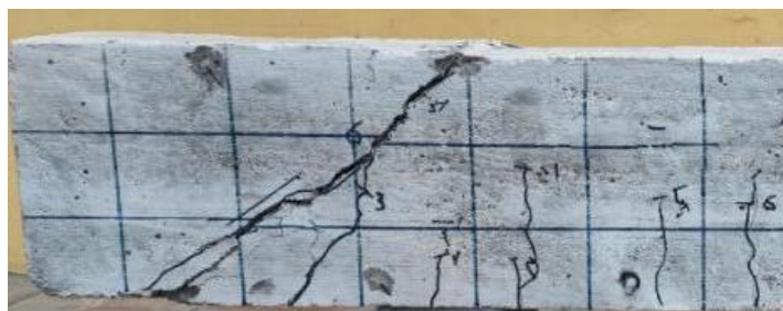
Figure 3. Formation of shear cracks in samples from the S1 series.
