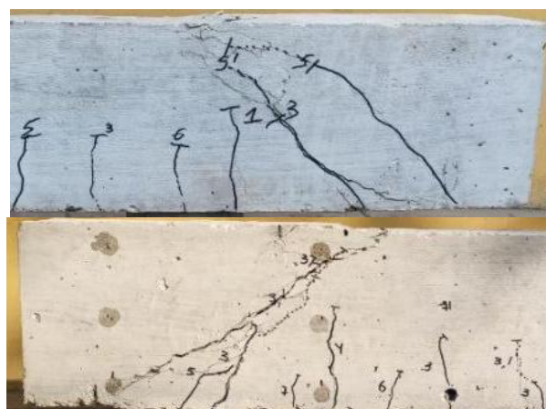
Figure 5. Formation of shear cracks in samples from the S3 series.
