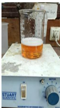
Figure 6. Preparation of selenium nanoparticles by reduction with Ascorbic acid.
