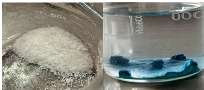
Figure 8. Extracted Dry Silica (Left) and NaOH/CuSO 4 Confirmation Test (Right).
