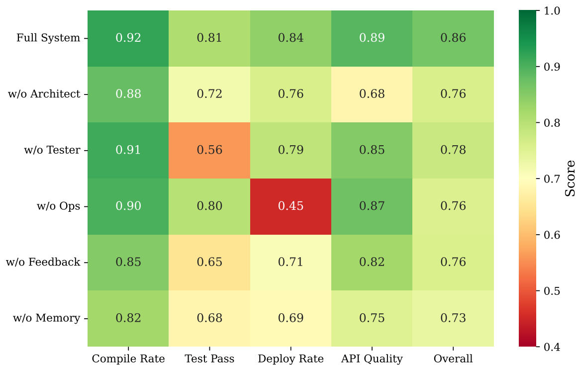
Figure 4. Ablation study results showing the impact of removing individual components. Darker green indicates higher scores; removing any component degrades overall performance. The Overall score is computed as the unweighted arithmetic mean of the four metrics (Compile Rate, Test Pass, Deploy Rate, and API Quality).
