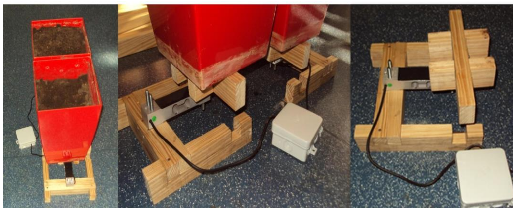
Figure 3. Precision weighing lysimeters mounted in a platform with load cells.
