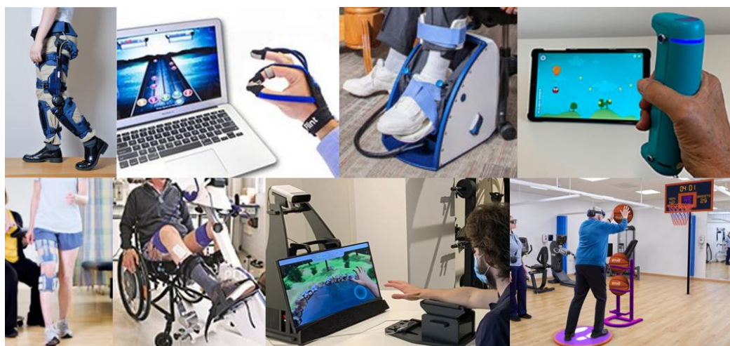
Figure 1. Representative examples of FDA-cleared rehabilitation devices suitable for home use after stroke. The collage shows one example device for each of the eight device categories used in this study. From top left to top right: actuated wearable ( Keeogo – B-Temia [40]), sensorized wearable ( MusicGlove – Flint Rehab [41]), robot ( Motus Foot – Motus Nova [42]), and exerciser ( GripAble Home – GripAble [43]). From bottom left to right: stimulator ( L300 – Bioness [44]), FES bike ( RT300 FES Cycle Ergometer – Restorative Therapies [45]), motion capture software ( RGS – Eodyne [46]), and VR/AR headset ( Reality DTx – Strolll [47]).
