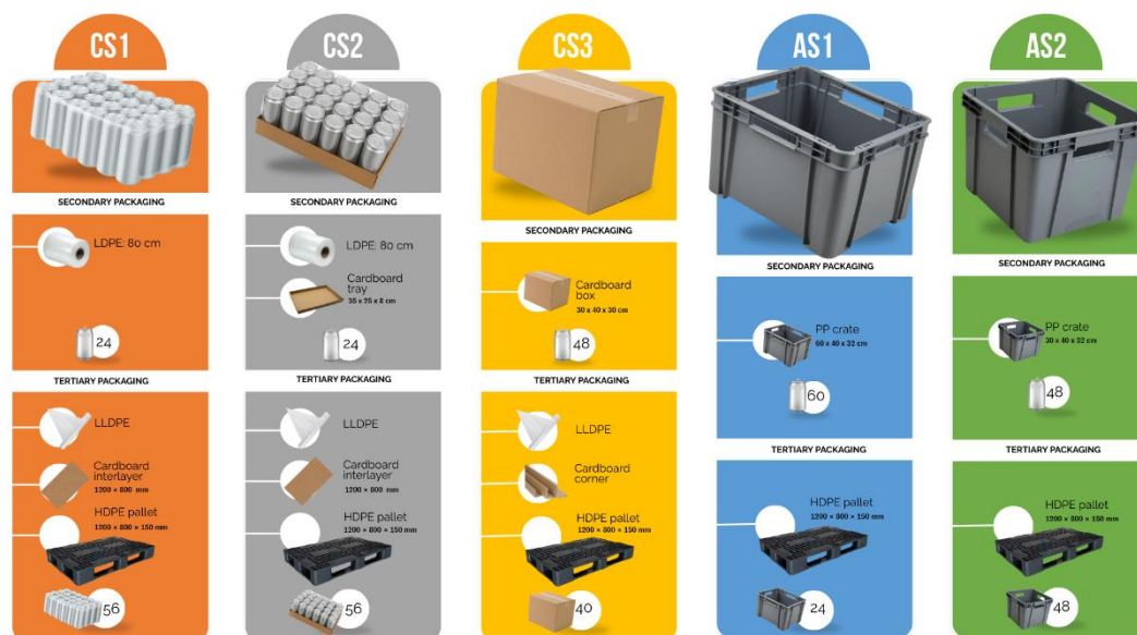
Figure 7. Secondary and tertiary packaging specifications for scenarios, including packaging type, component dimensions, unit capacity, and number of units per secondary packaging and pallet. Acronyms: CS: Current Scenario; AS: Alternative Scenario.
