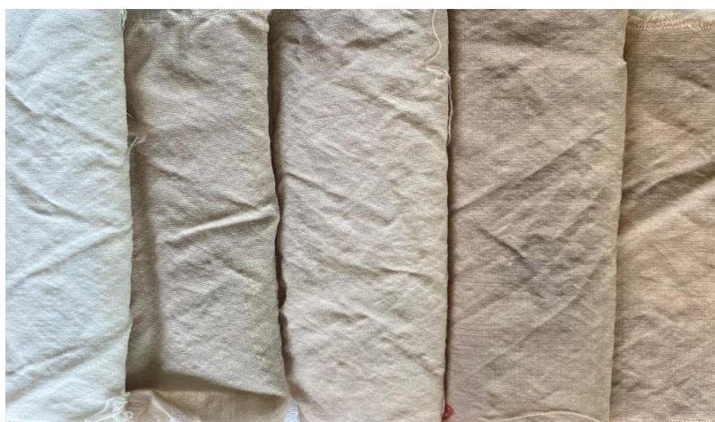
Figure 5. Wool fabric dyed with protein hydrolysate from BSF cocoons without mordant; dye protein concentration 2%, 5%, 10%, 30%, 50% w/w o.w.f. from left to right.
