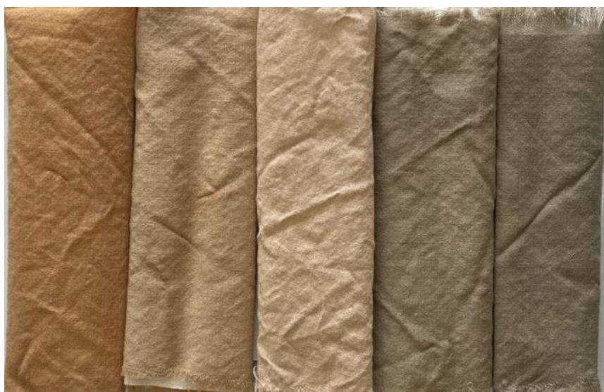
Figure 7. Wool fabric dyed with protein hydrolysate from BSF cocoons with 5% o.w.f. mordant; dye protein concentration 2%, 5%, 10%, 30%, 50% w/w o.w.f. from left to right.
