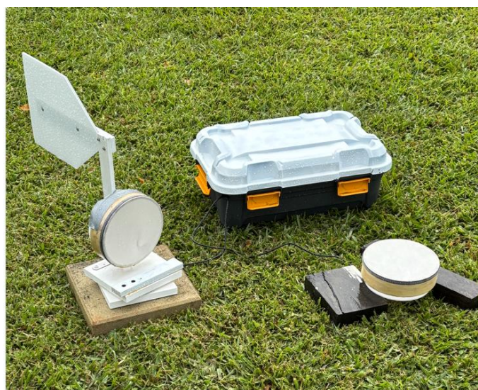
Figure 1. Photo showing the acoustic sensors (vertical sensor on the left, mounted on the wind vane) and horizontal sensor on the right. The weatherproof case at rear holds the power supply and the microcontroller and data logging system.
