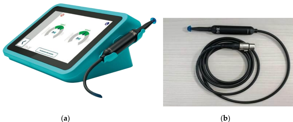
Figure 1. (a) Measurement device Medwave to perform the analysis of the functional status of the middle ear using the PLAI (Pressure Less Acoustic Immittance) method. (b) Probe of the Medwave® device with an earplug. (The copyright of this figure belongs to Neuranix Srl, Gardigiano di Scorze, Italy).
