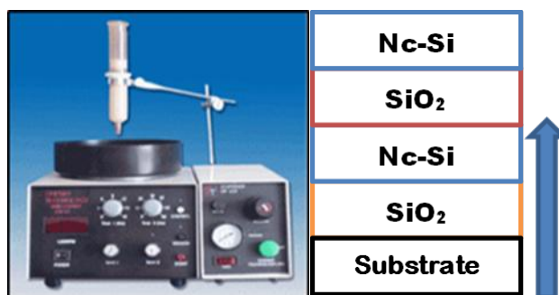
Figure 1. (a) Schematic diagram of the Spin coater set up and (b) Cross-sectional diagram of MLnc-Si/Si thin film growth.
