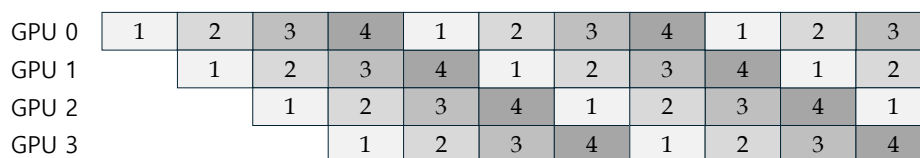
(a) Ideal Pipeline: balanced micro-batch workloads, no idle.
