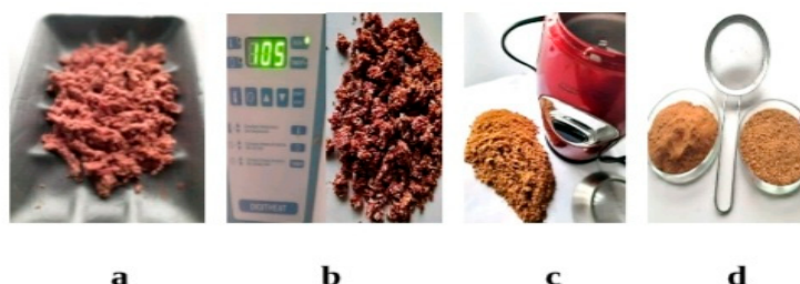
Figure 4. Crude insoluble residue and intermediate and final products of its transformation: a -crude residue; b -dried residue, c - dried residue after grinding; d - two fractions from the separation of the crushed residue on a sieve with 0.5 mm holes.
