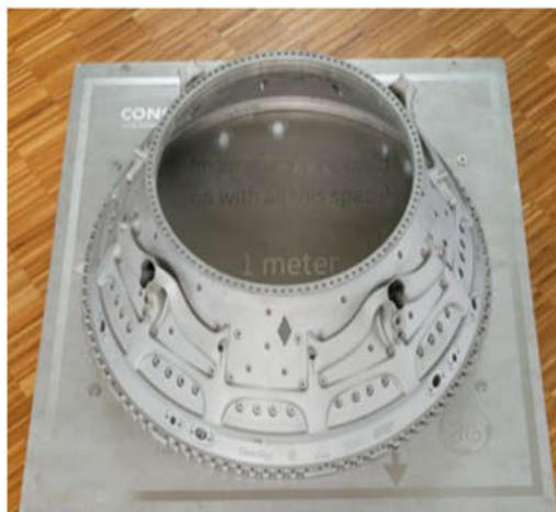
Figure 3. A representative aerospace component fabricated by metal additive manufacturing using the nickel-based superalloy Inconel 718 (courtesy of GE Aerospace), illustrating design consolidation, weight reduction, and suitability for high-temperature structural applications where complex geometries and performance-driven optimization are required [37].
