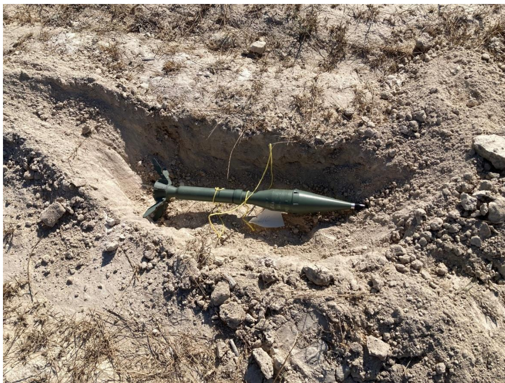
Figure 3. (a) Set of metallic cylindrical objects used in the experimental campaign to simulate buried UXO. (b) 105 mm projectile and detail of its placement in the ground during the test. (c) 20 mm mortar round placed in a vertical position for data collection. (d) 155 mm projectile and detail of its placement in the ground. (e) 60 mm mortar round and detail of its placement in the ground. (f) Details of the placement process for the negative-control anti-tank projectile.
