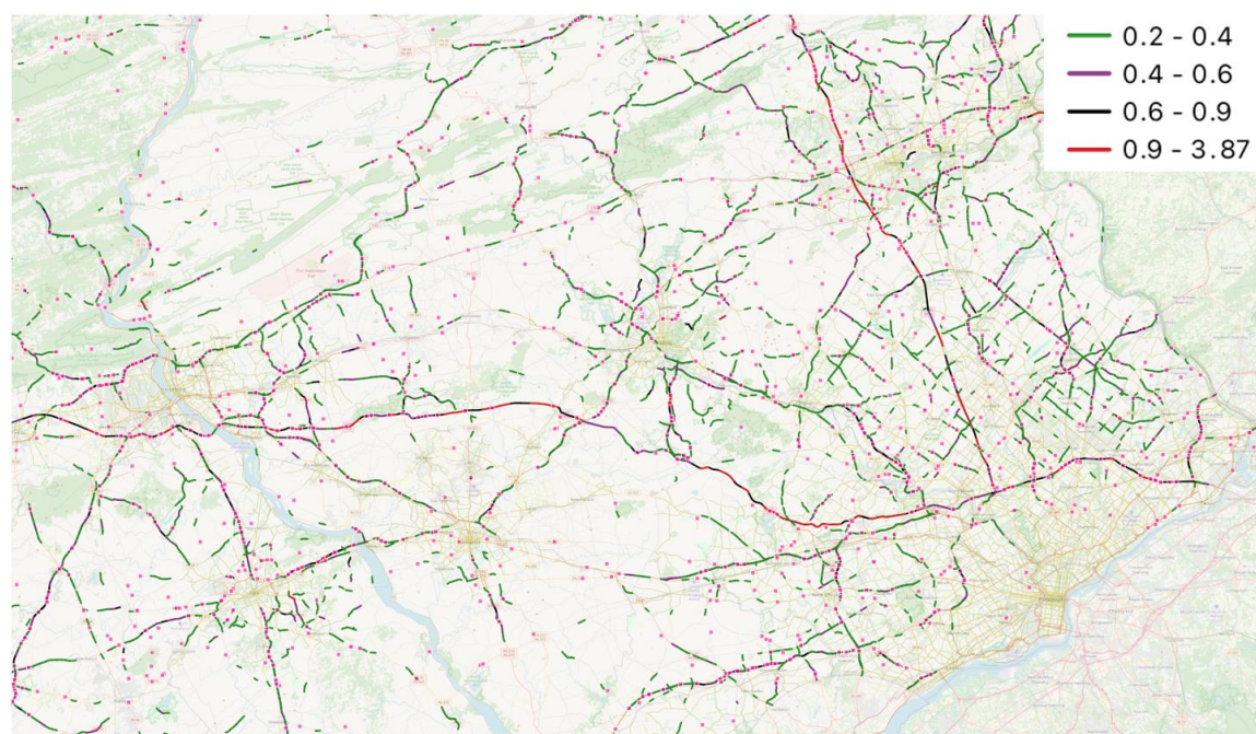
Figure 5. Model Performance Across Segment-Quarter Risk Classes: Predicted and Observed DVC Counts for Q4 2024 in map between Harrisburg and Philadelphia.
