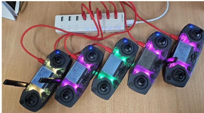
Figure 8. Drone controllers are connected to the port hub.
