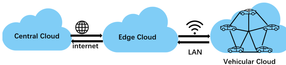
Figure 1. Vehicular networks architecture
