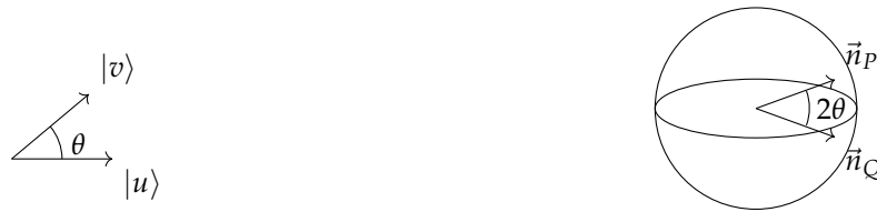
(a) Principal angle \theta between rank-1 projectors ( P = |u\rangle\langle u| , Q = |v\rangle\langle v| ). (b) Bloch-sphere rendering: axis difference equals 2\theta .
