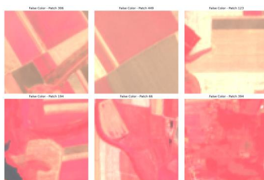
Figure 4. Sample patches showing false-color composites (bands 8–4–3, NIR–Red–Green) for soil and vegetation classes. Vegetation is enhanced in red tones, aiding class discrimination.
