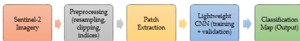
Figure 2. Workflow of the proposed classification pipeline, including preprocessing, patch extraction, CNN training, and evaluation.
