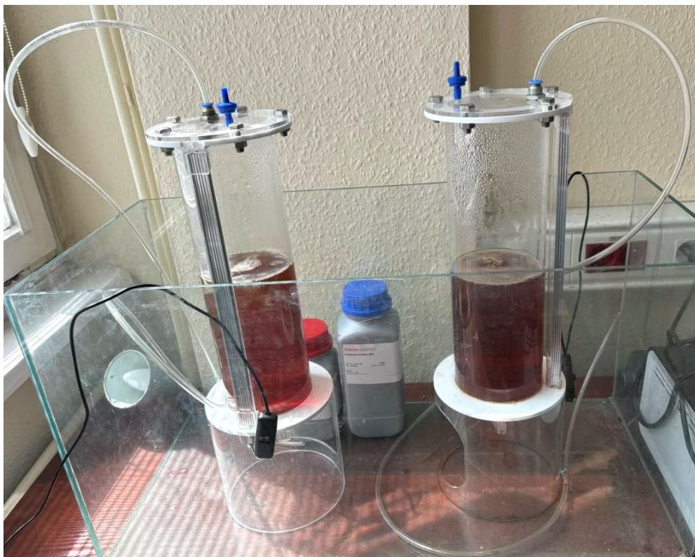
Figure 1. Experimental setup for testing kombucha-PBR system. Two bioreactors were filled with wastewater with microbial kombucha consortium.
