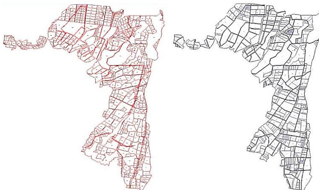
Figure 4. Cadastral Parcel Layouts in Büyükkoba Village, Kırşehir Province, Before and After Land Consolidation.
