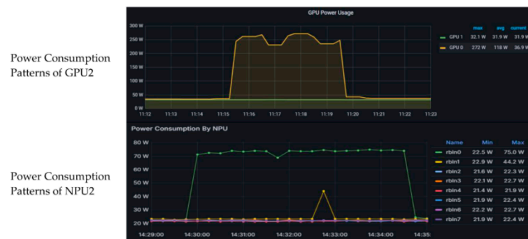
Figure 3. Power consumption patterns of GPU and NPU accelerators under sustained streaming workloads.
