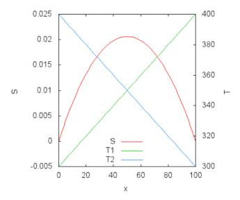
The change in temperature is shown on the right axis of the ordinate:  $T_1 = 300 + x$ ,  $T_2 = 400 - x$ , the change in entropy on the left. The entropy reaches the maximum value at x = 50 when the temperatures of the subsystems become equal.
