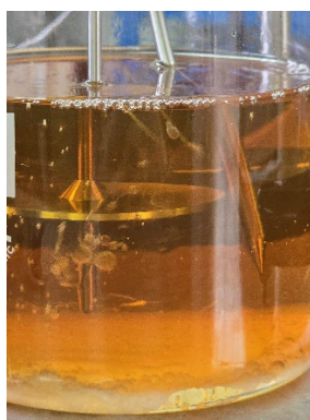
Figure 1. Appearance of the emulsion formed by water in engine oil.
