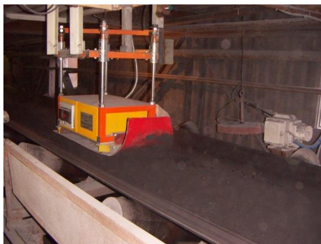
Figure 9. Online XRF analyzer on an iron-ore mixture conveyor.
