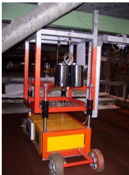
Figure 11. Online XRF analyzer on the belt filter with iron-cake.
