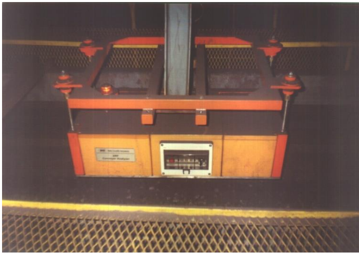
Figure 14. Online XRF analyzer above the conveyor with Vanadium Slag.
