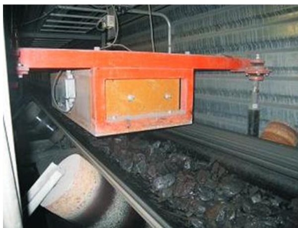
Figure 3. Online XRF analyzer on a standard suspension on four legs above the conveyor belt.
