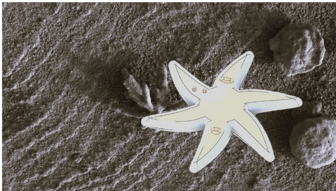
Figure 1. Artistic rendition of a soft robotic Total Habitability Instrument (THI) measurement system for planetary exploration. Capable of measuring conditions for habitability such as ions, water CHNOPS.
