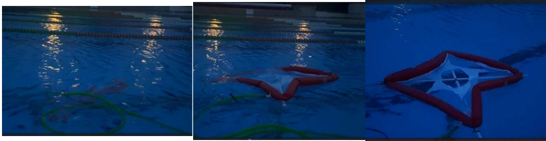
Figure 4. The operating stages of the airbag mechanism from its placement under water to its exit from the water surface.
