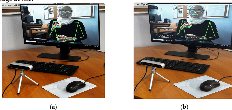
Figure 3. Experimental setup with a user signing in ASL. The video feed with overlaid keypoints is displayed on screen. (a) A status message is displayed during inference; (b) The translated text is displayed once inference is complete.
