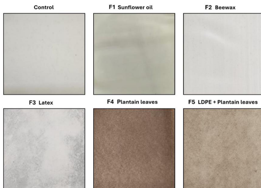
Figure 2. Images of films extruded by flat sheet extrusion for different compounded TPS formulations.
