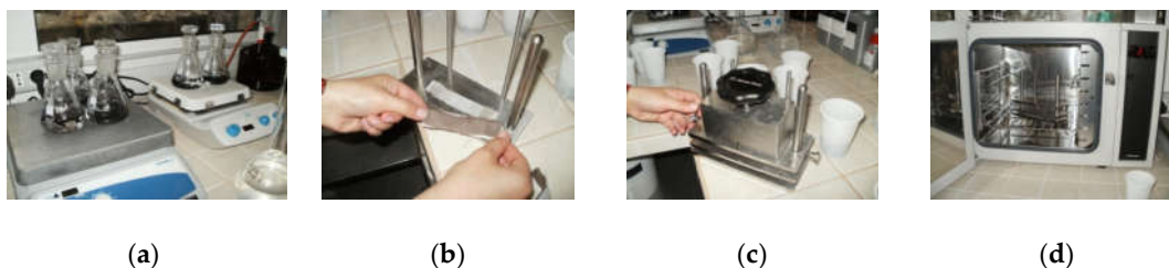
Figure 5. Perspiration fastness testing: (a) impregnation of samples; (b) sample placement; (c) applying pressure; (d) HX30 model oven.
