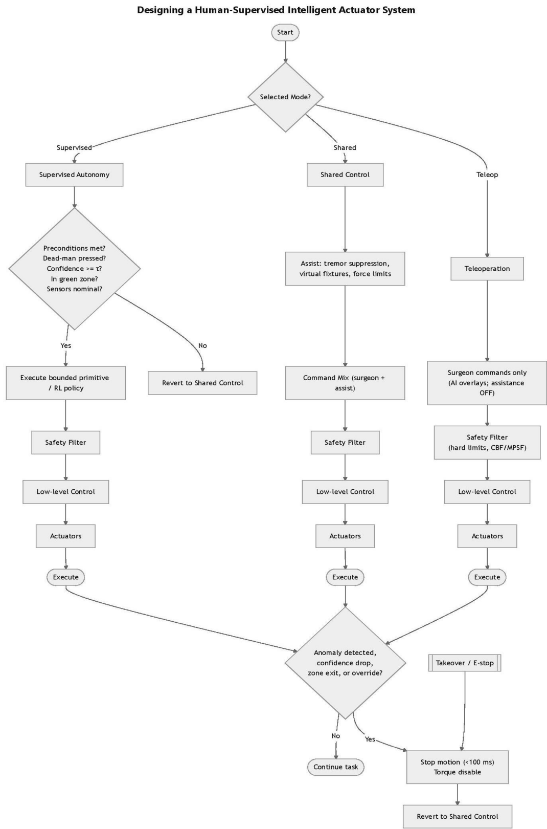
Figure 1. Flowchart of the Proposed Human-Supervised Intelligent Actuator for Minimally Invasive Surgery.
