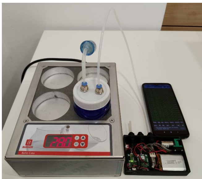
Figure 1. Prototype electronic nose equipped with MOS sensors.
