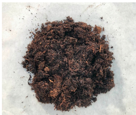
Figure 1. Appearance of factory-derived tea waste, consisting of leaf residues, fibers, and fine particles excluded during the processing of green tea into black tea.
